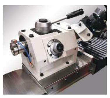
Manual lever movement and push with adjustable preload spring, with Morse 3 connection (optional Morse 4). The sleeve, sliding on adjustable bushings, can have a pneumatic opening and closing movement to facilitate the loading and unloading of the pieces. The fine adjustment of the cylindricity, equipped as standard in the tailstock, can be motorized and managed by the NC, to reduce the machine alignment time. Programming is done by directly entering the correction value in a specific CNC mask.
