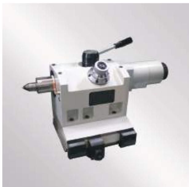
The **X1000** tailstock unit has everything you need: movement manually controlled by lever or automatically by pedal; the centre pressure can be adjusted by spring or hydraulic force. The cylindricity correction of the pieces is made by a practical knob equipped with an optical scale. The movement of the group along the table takes place through a rack that facilitates the operator in the setup operations.
