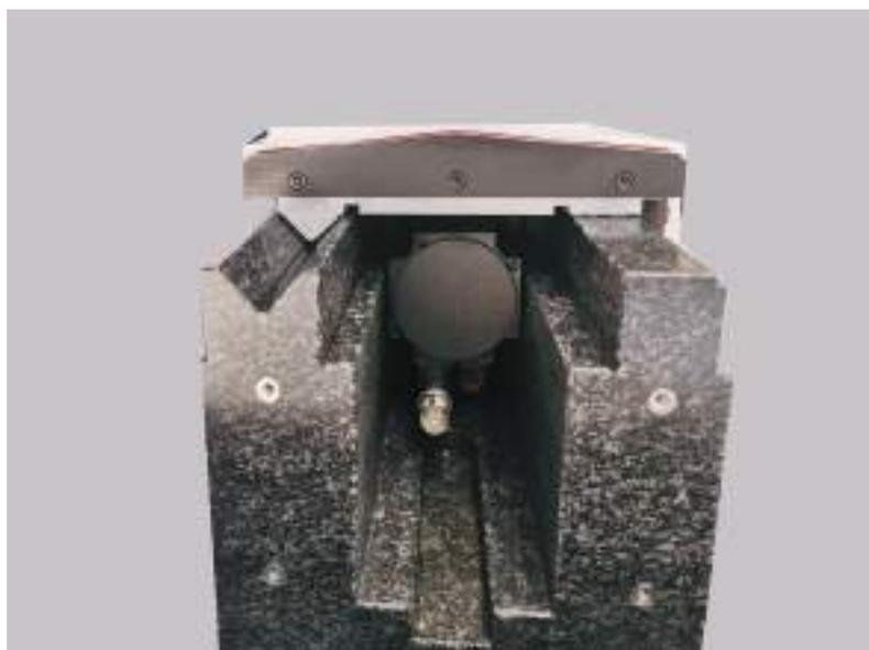
The flat-prismatic sliding of the table, with the interposition of anti-friction material, is made directly on the granite base. The wheel-holder carriages run on linear guides with recirculating roller and all axes are controlled by pressurized absolute optical scales.
